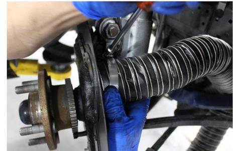
Step 27) Route the tubing as shown (this routing can vary depending on what you have to work with) and use one of the big clamps to secure the middle of the tubing where you can. Each side. (see images 4 and 5)
