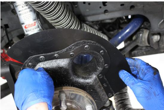
Step 23) Cut brake duct tubing in half using a razor blade and dikes. Be sure edges are somewhat "cleaned up" so not to cut yourself with the sharp ends.
