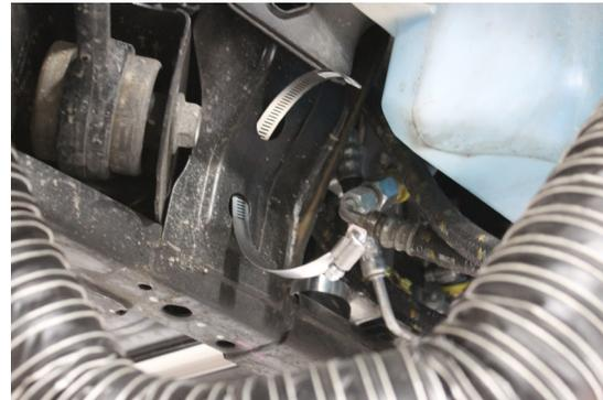
Step 28) Test to ensure the tubing does not bind or pull on the clamps by turning the wheel all the way to the left, then all the way to the right. If binding or pulling happens, adjust the routing, re-secure tubing, and re-test. Each side.
