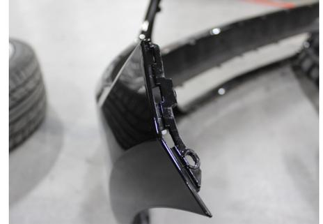
Step 11) Remove the fog lamp/turn signal housing from the backside of the fascia by removing the (6) 7mm bolts (see image 4). (2) of these have washers. Note the location where these (2) were removed from as they will need to go back to those same locations. Now, using a flat head screwdriver, release the tabs that hold the housing in place, starting at the outside tabs and working your way in. Each side.
