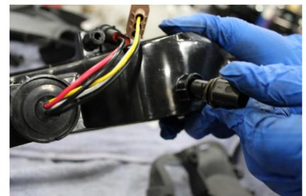
Step 13) Remove the (3) 7mm bolts from the housing that secure the turn signal lamp. Each side. (see image 6)
