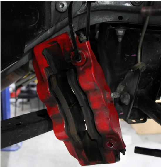
Step 19) Remove brake caliper by removing the (2) nuts holding it in place (nuts and location will vary depending on brake system). Each side.
